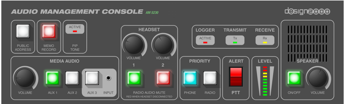
Figure 5.1.1 – AMC Front Panel Diagram
